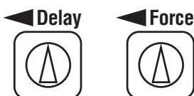
Turn the corresponding regulator clockwise to increase the parameter.
